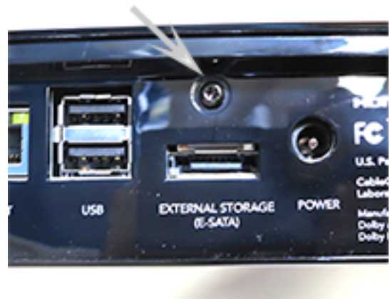
Figure 2 - One screw to remove
