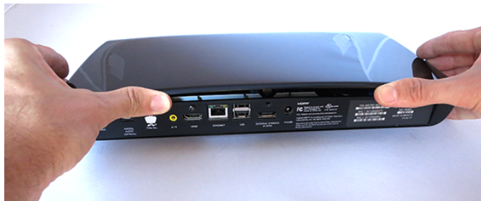
Figure 3 - Removing the TiVo Roamio top cover
