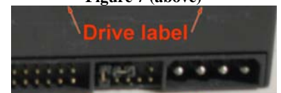
Two-jumper Maxtor Set as “Master”
