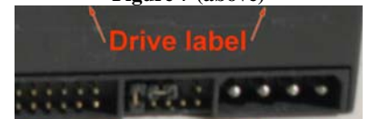
Two-jumper Maxtor Set as “Master”
